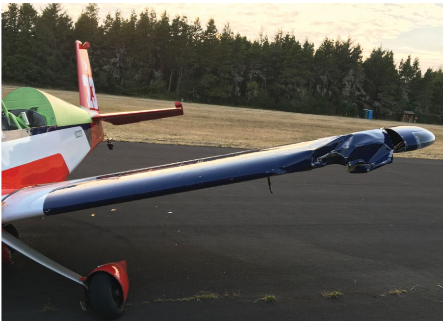
Here you can see where the second elk struck the wing, spinning the aircraft around and causing the landing gear to snap. Thankfully, neither the pilot nor his passenger were injured, but the plane was declared a total loss. Photos provided courtesy of Todd Rudberg
