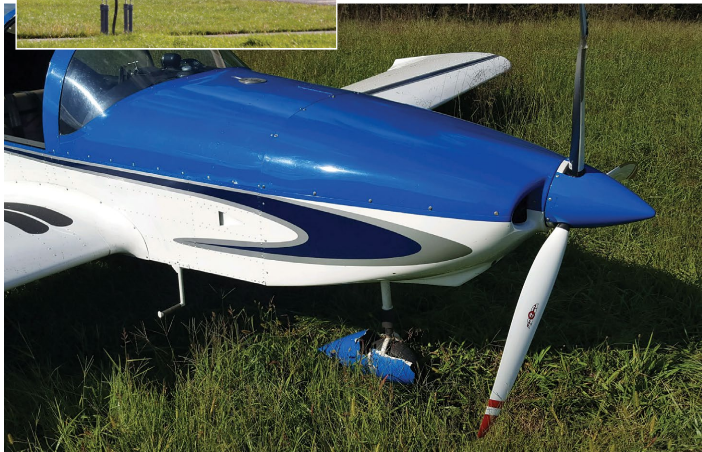
This 2008 Breezer's nose pants were destroyed and its nose wheel steering rods were seriously damaged when it struck a deer while landing. The left wing flap and leading edge were also damaged. Photos provided courtesy of Arthur "Bo" Mills
